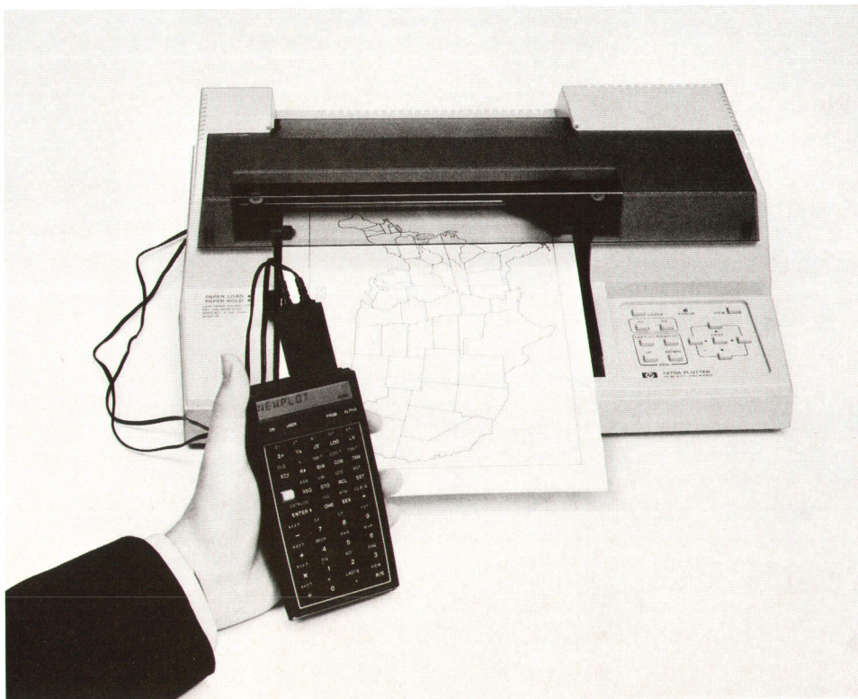
Fig. 1. The HP 82184A Plotter Module and HP 82160A HP-IL Module are easily inserted into two of the four I/O ports at the top of the HP-41C Programmable Calculator, providing low-cost graphic output to an HP 7470A Graphics Plotter.
